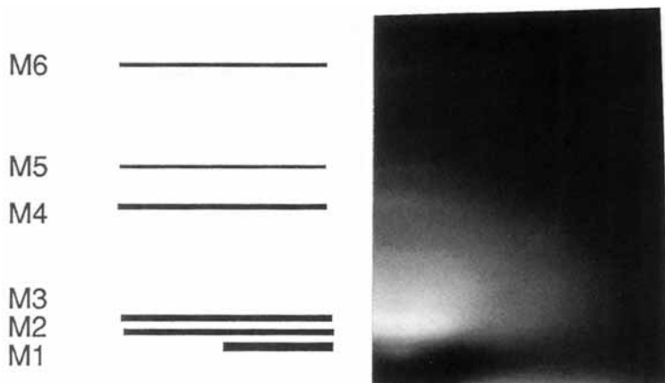
Fig. 2. WAXS print of PBZT coagulated in iodine/ethanol, spin/draw = 9.7 [PI9]. Meridional reflections are emphasized.
